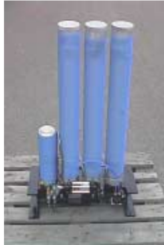
Filter panel with autodrain for Swedish Navy.
